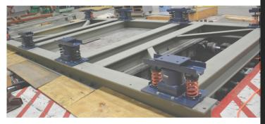
TRU Compliance, through its affiliate Seismic Test Co., has a dedicated shake table. The 10'x10' table can test equipment up to 10,000-lbs. in base, wall, and ceiling mounted configurations.
